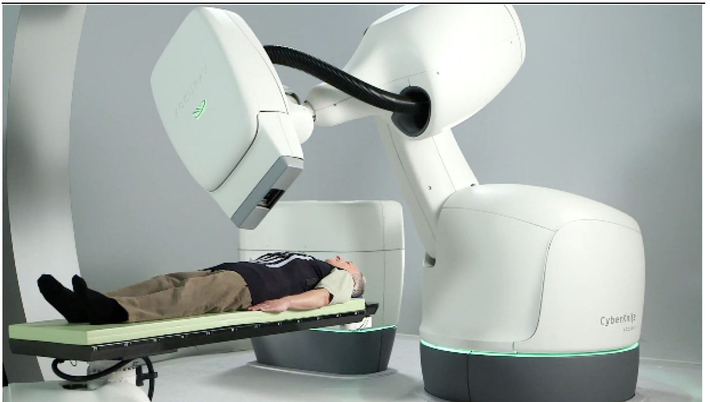
Figure 3. The CyberKnife® M6™ robotic radiosurgery system displaying the robotic manipulator, robotic couch, and the InCise multileaf collimator.
